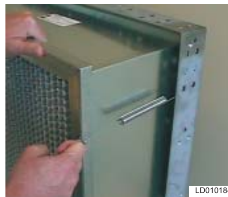
FIG. 43 – SPRING LATCH SHOULD BE PULLED AND FASTENED IN HOLE IN THE HEADER OF THE FILTER.
