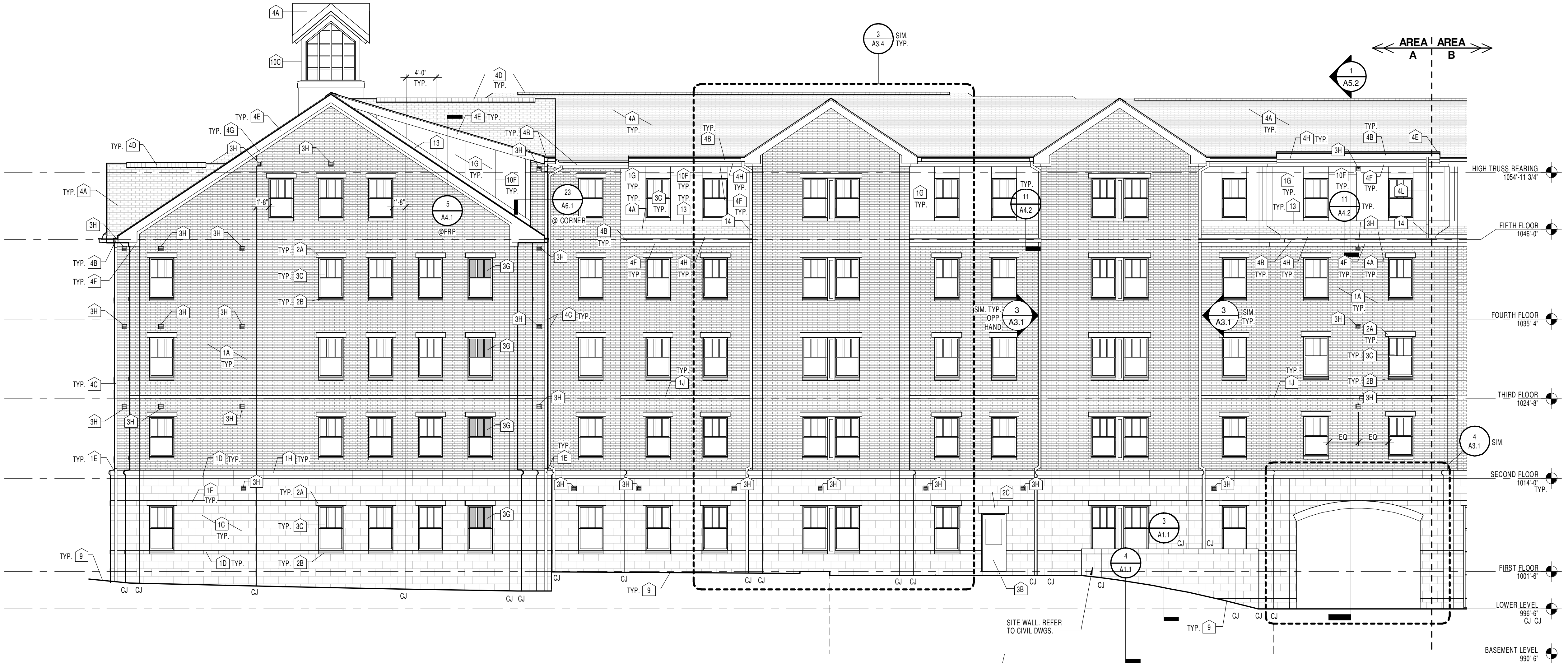
1 EAST BUILDING ELEVATION - AREA A 1/8" = 1'-0"
