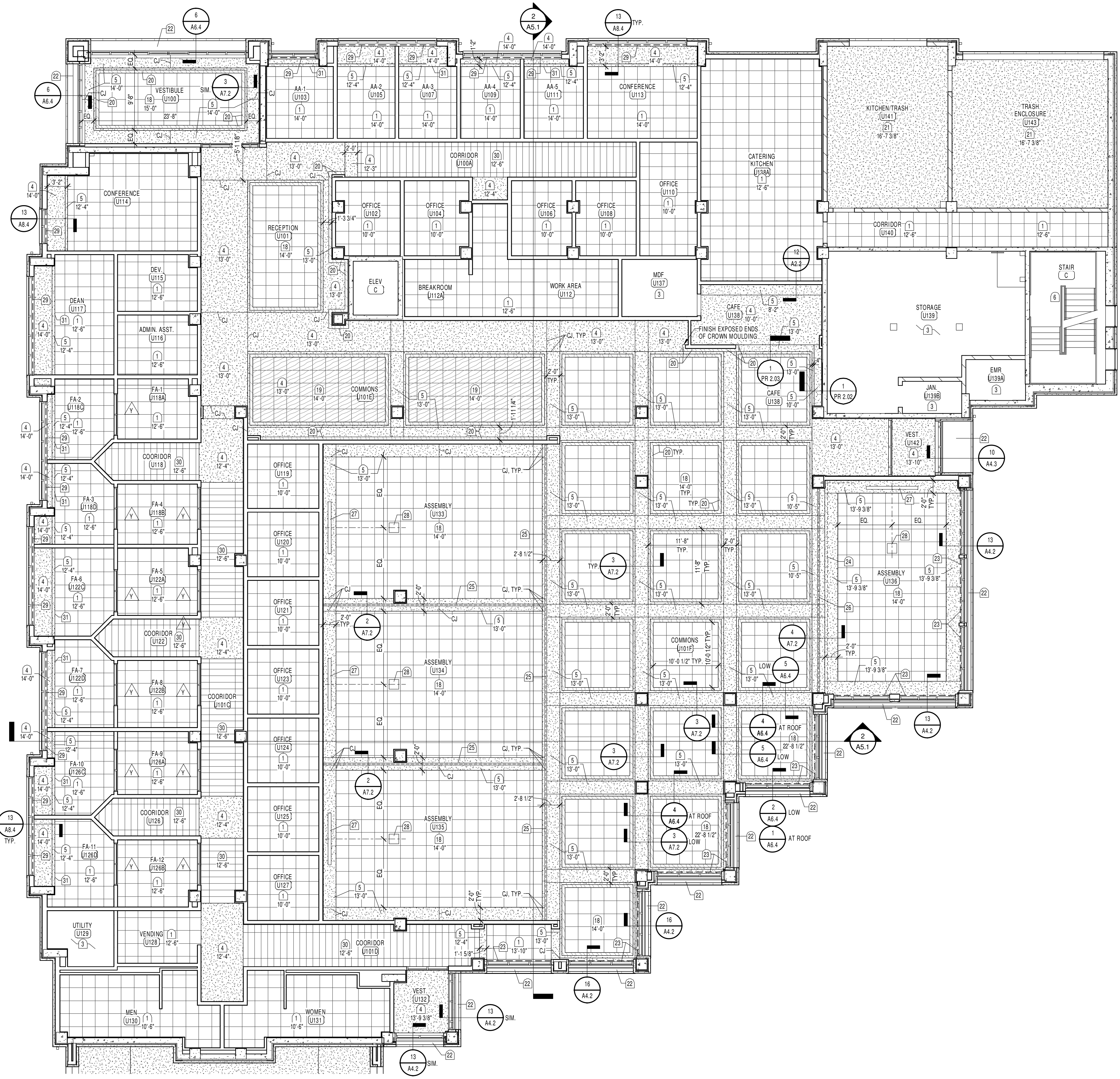
1 LOWER LEVEL REFLECTED CEILING PLAN - AREA B 1/8" = 1'-0"
