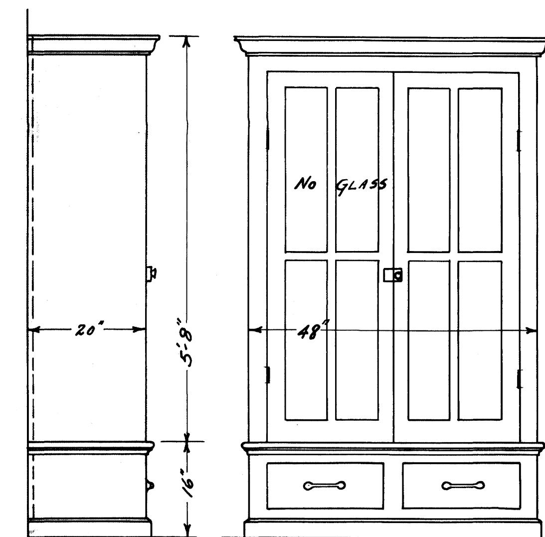
DETAIL 57. SCALE 3/4"=1' OAK, VARNISHED. 2 WANTED. 57-A. 2 WANTED WITH GLASS AND 4 ADJUSTABLE SHELVES.
