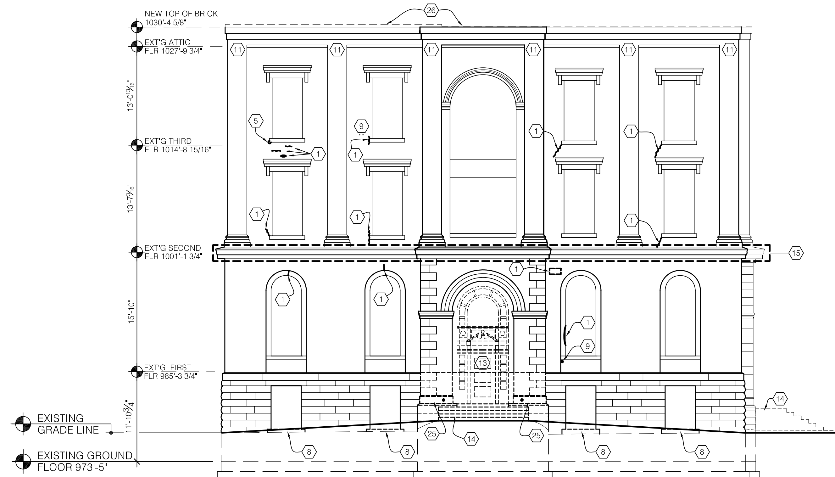
DEMOLITION & MASONRY REPAIR - NORTH ELEVATION
