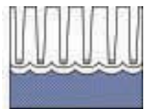
2 - Color added to bottom of coating pores.
