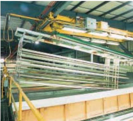
Aluminum extrusions are lowered into the anodizing tank
