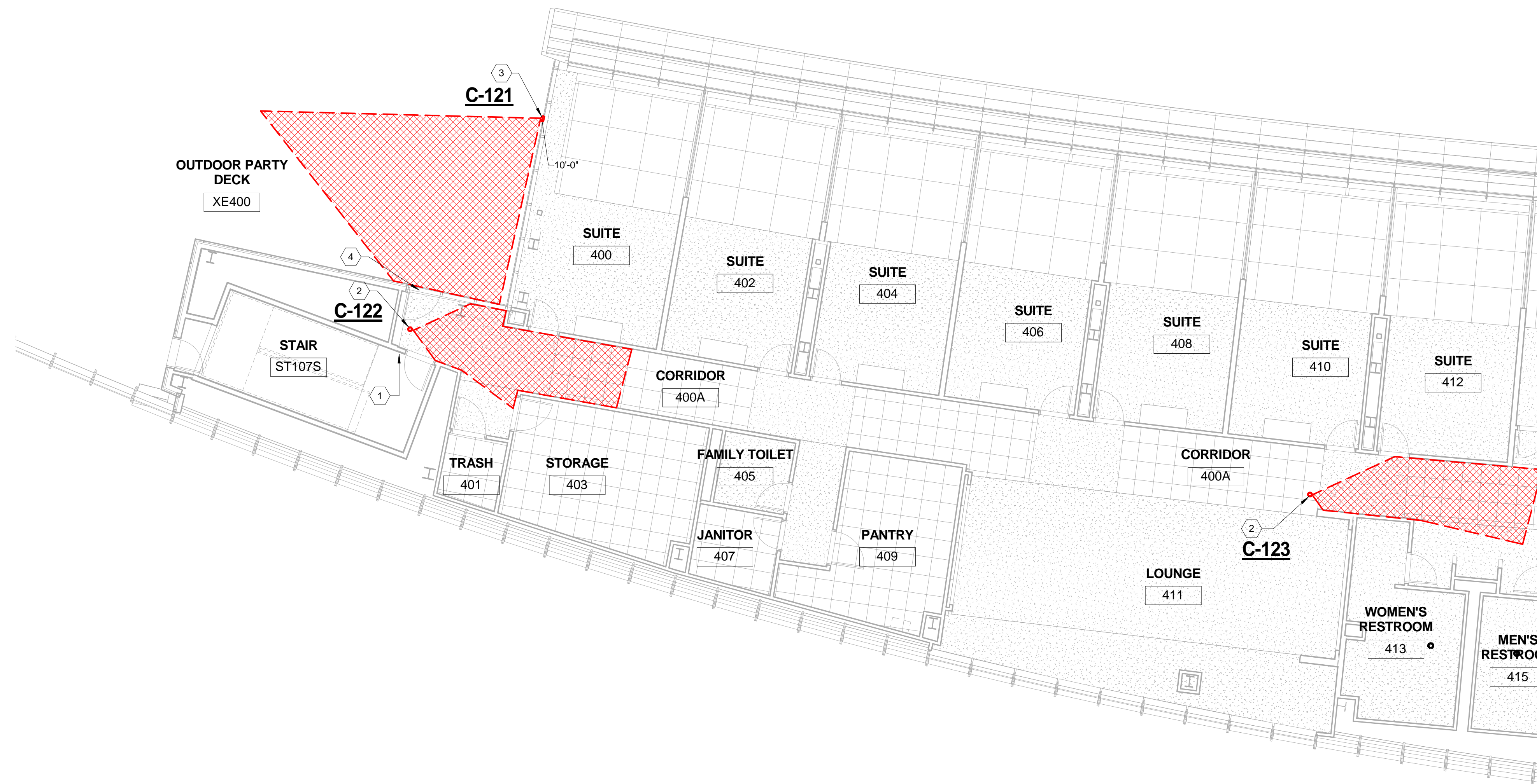
① SUITE LEVEL ELECTRONIC SAFETY & SECURITY PLAN - S1 1/8" = 1'-0"
