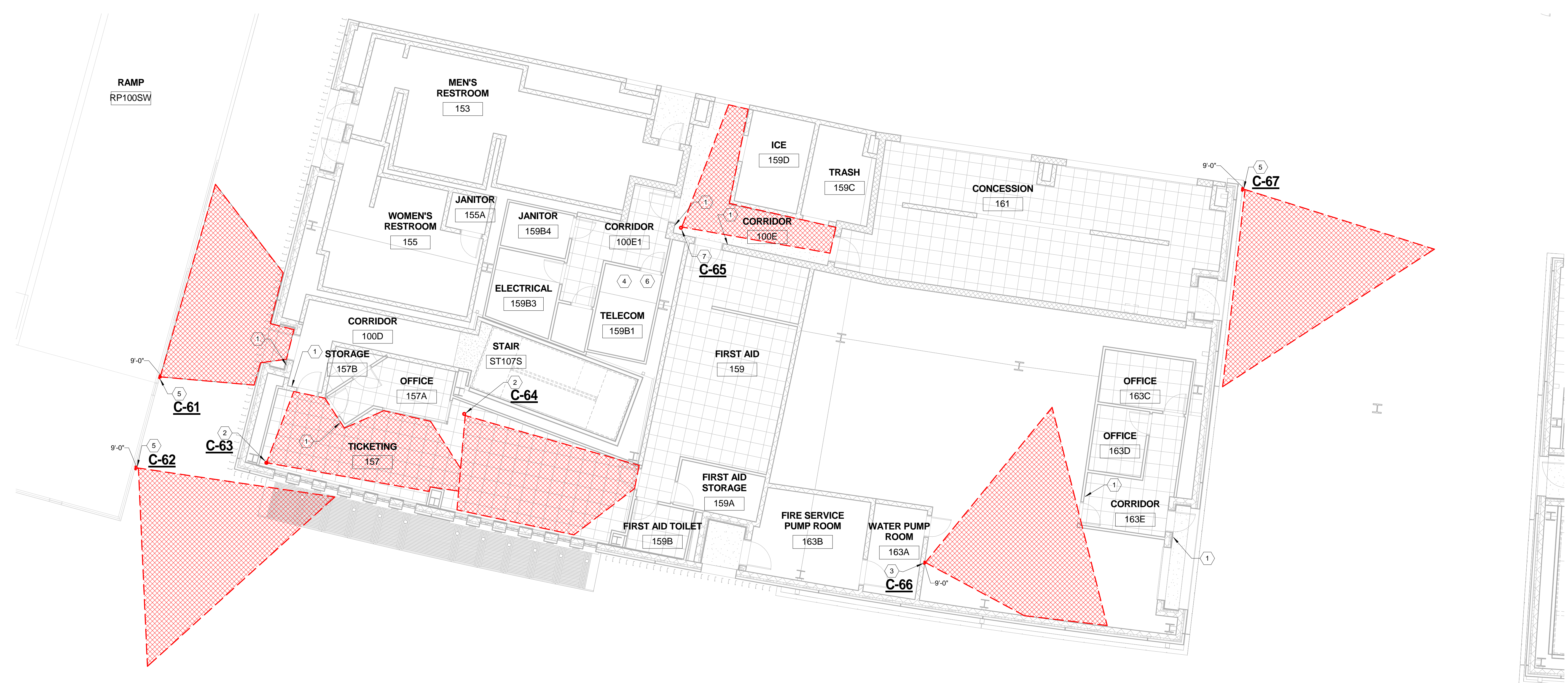
1 MAIN CONCOURSE ELECTRONIC SAFETY & SECURITY PLAN - S1 1/8" = 1'-0"
